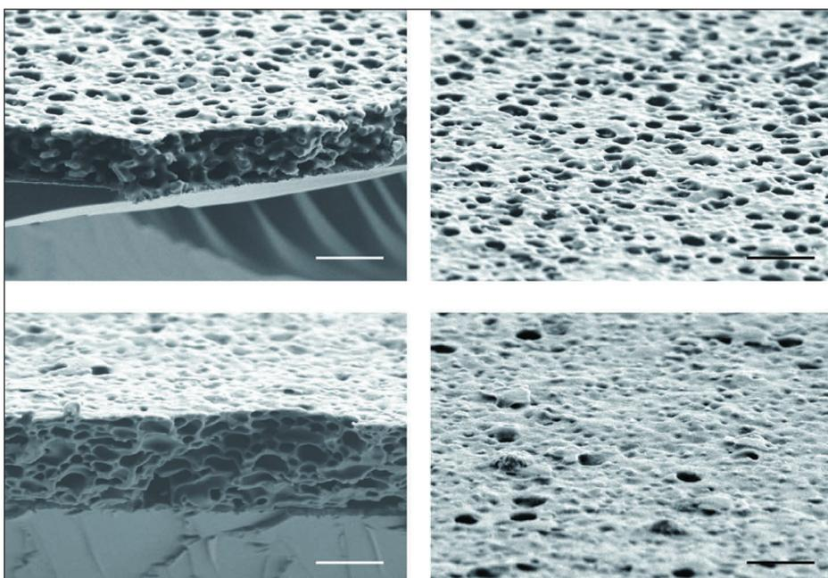
Figure 2. Cross-sectional and surface SEM images of porous membranes after oxidation (*top*) and reduction (*bottom*) (scale bar: 1 µm).
