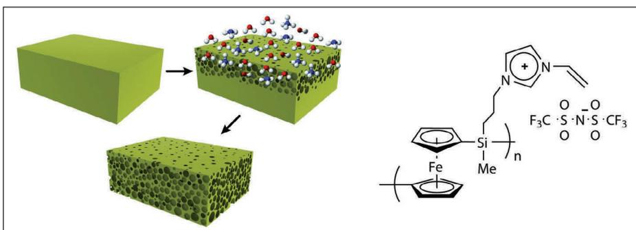
Figure 3. Representation of the pore-formation process induced by ammonia diffusion (*left*); chemical structures of poly(ferrocenylsilane)-based poly(ionic liquid) used in this study.
